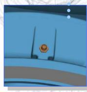
From size 180 and up all motors are equipped with a greaser
